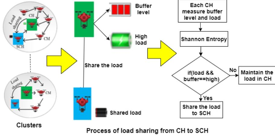
Figure 4.3: Entropy based Load Balancing
