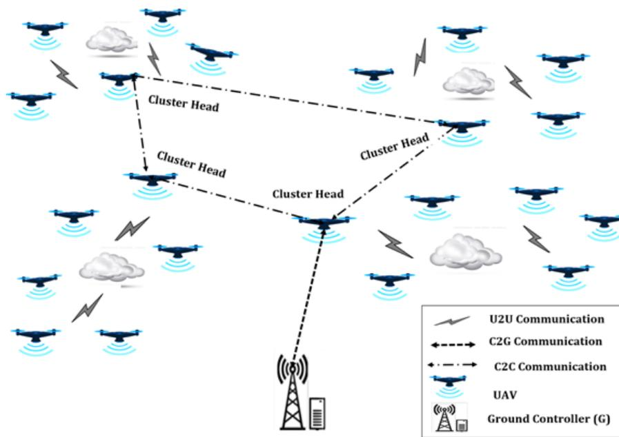
Figure 3.3: Cluster-based ad hoc interactive deployment.
