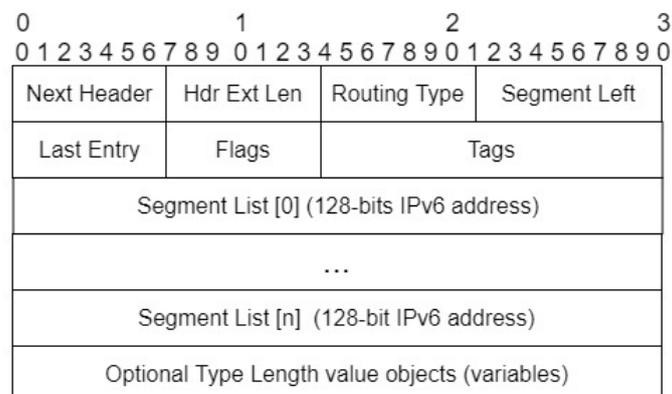
Figure 5.1: Segment Routing Extension Header
