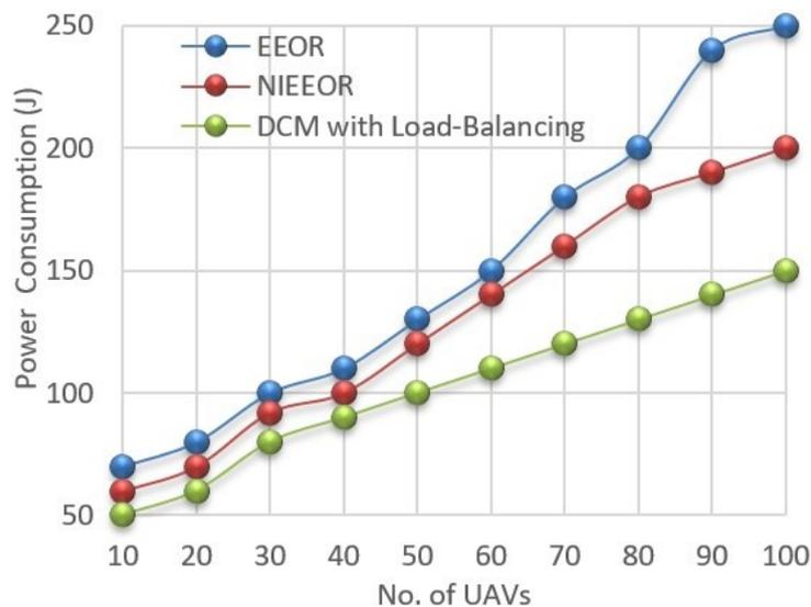
Figure 4.8: Number of UAVs vs. Power consumption
